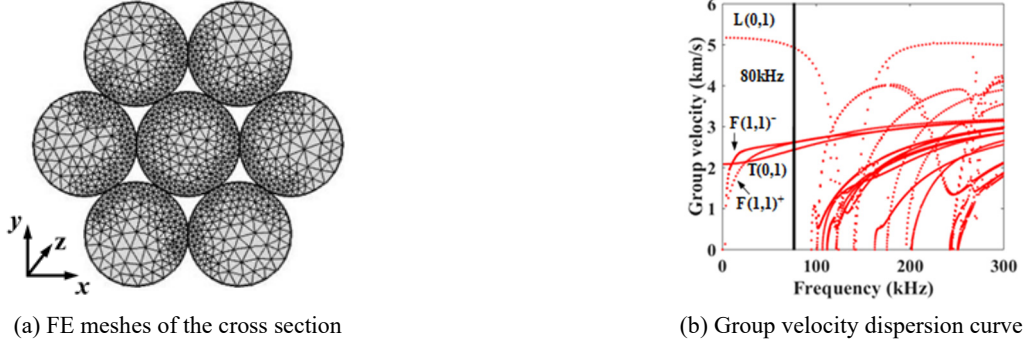
Fig. 1 Dispersion analysis results of the seven-wire steel strand
