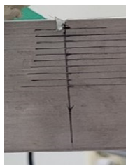
Fig. 18 Inflicted crack ( a/h = 0.085 )
