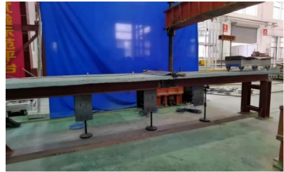
Fig. 23 Test beam system using three PTMD devices
