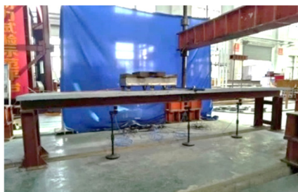
Fig. 19 Placement of the whole test system using a simply supported beam
