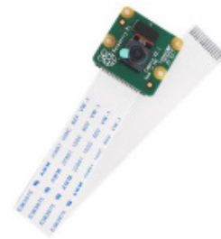
Fig. 2 Photography module Raspberry Pi camera v2
