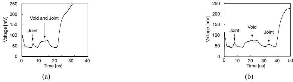
Fig. 8 TDR waveform measured in concrete block using transmission line with joint: (a) case 1; (b) case 2
