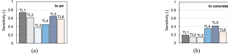
Fig. 6 Sensitivity of transmission lines with different configurations: (a) in air; (b) in concrete
