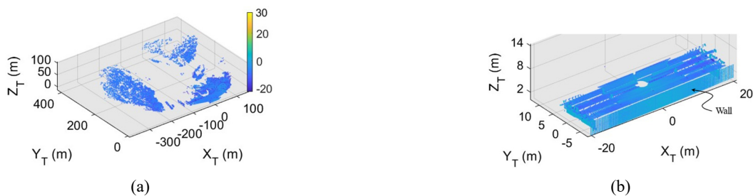
Fig. 3 (a) Raw point cloud and (b) background filtered point cloud showing the ROI of the bridge girder
