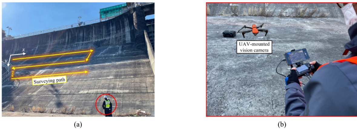
Fig. 5 Target in-situ dam structure: (a) Pre-defined surveying path; (b) UAV-mounted vision camera
