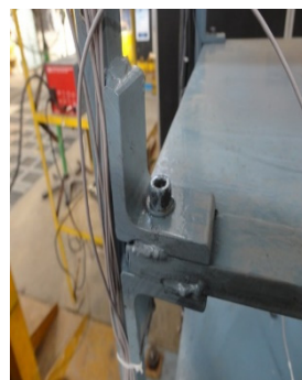
(b) Column & plate connection detail
