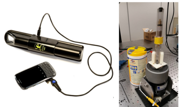
Fig. 6 nPower PEG as sold (left) and with protective case removed and mounted on a shaker to retrieve experimental data (right)
