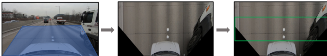
Fig. 5 Captured images using IMP: (a) Raw image in which the blue box corresponds to RoI; (b) Bird's-eye view by IMP; (c) RoI marked with a green rectangular box
