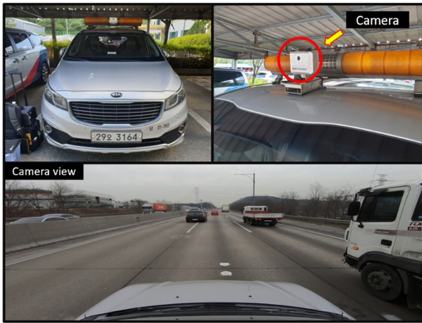
Fig. 1 Camera-mounted Road inspection vehicle and its camera view
