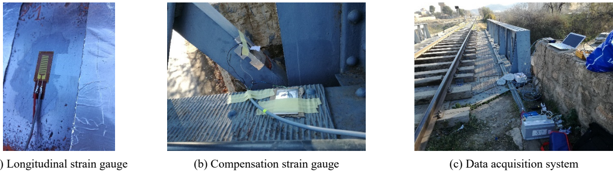
Fig. 4 Experimental strain measurement
