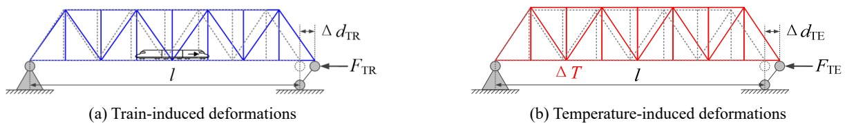
Fig. 12 Illustration of bridge deformations
