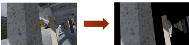
Fig. 3 An example of our semantic-guided masking module. Non-column regions are replaced with black
