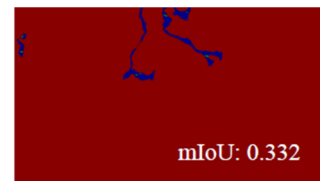
(c) Pure texture damage segmentation
