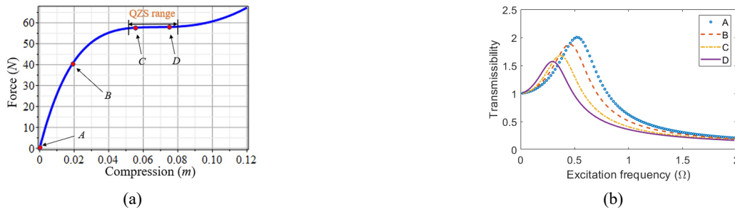
Fig. 16 Isolation performance with the QZS effect: (a) optimal static force with enlarged QZS range and (b) the transmissibility curves with different working positions
