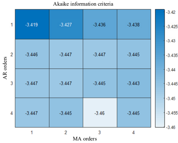
Fig. 13 The instance for calculated AIC value to select a suitable model order
