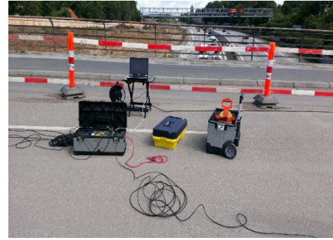
Fig. 7 DAQ toolbox (NI 9233)
