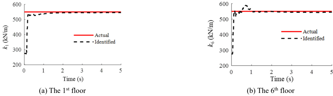
Fig. 2 The identified stiffness of shear building structure
