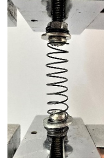
Fig. 5 Tensile test of SMA spring
