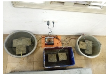
Fig. 4 Concrete with sensor embedded immediately after casting
