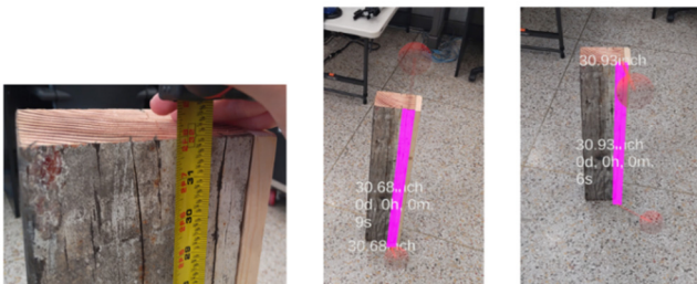
Fig. 9 Traditional measurement of feature versus measurement with the AR measure function, taken from top to bottom and bottom to top respectively
