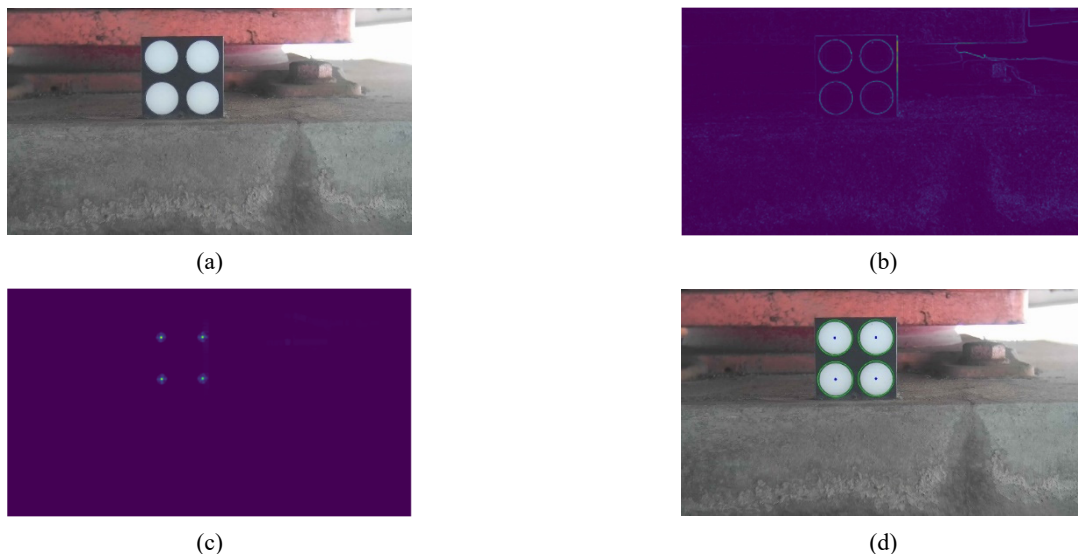
Fig. 8 Circular Hough transformation examples: (a) Original image; (b) Sobel edge detection; (c) accumulator array computation; (d) center and radius estimation
