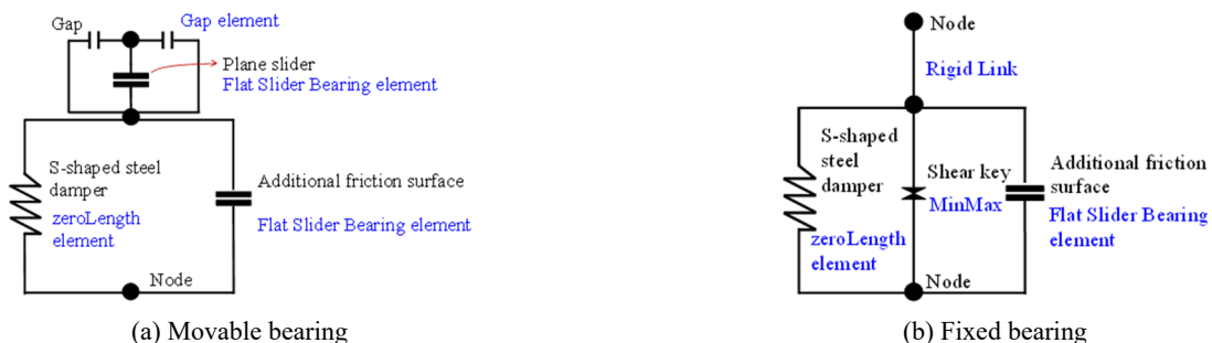
Fig. 20 Numerical model of SSDFB in OpenSees
