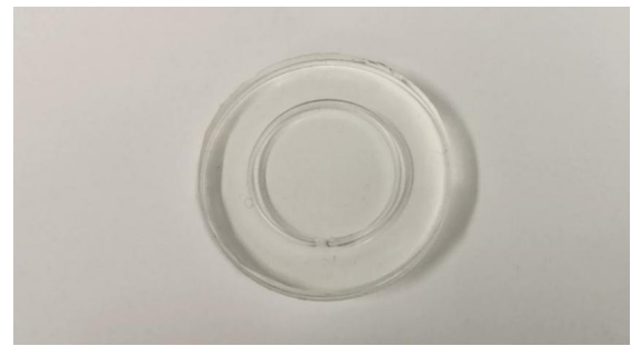
Fig. 14 The finished PDMS substrate
