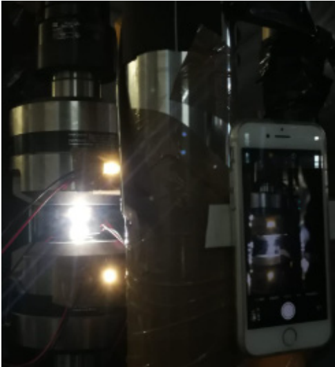
Fig. 5 Four markers are glued on the machine-specimen system
