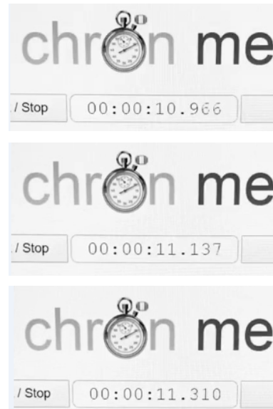
Fig. 6 Video progress for checking the actual frames per second rate: (a) images 1 and 5; (b) image 9
