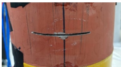
Fig. 9 Inflicted crack ( \theta = 23.72^\circ )
