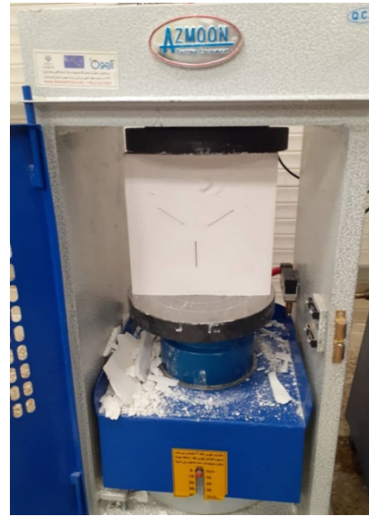
Fig. 7 Specimen are placed between the plates of the loading machine
