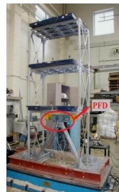
Fig. 25 The 1/4 scale, 3-story steel frame
