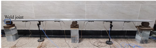
Fig. 34 The overall placement of the tested two-span continuous beam
