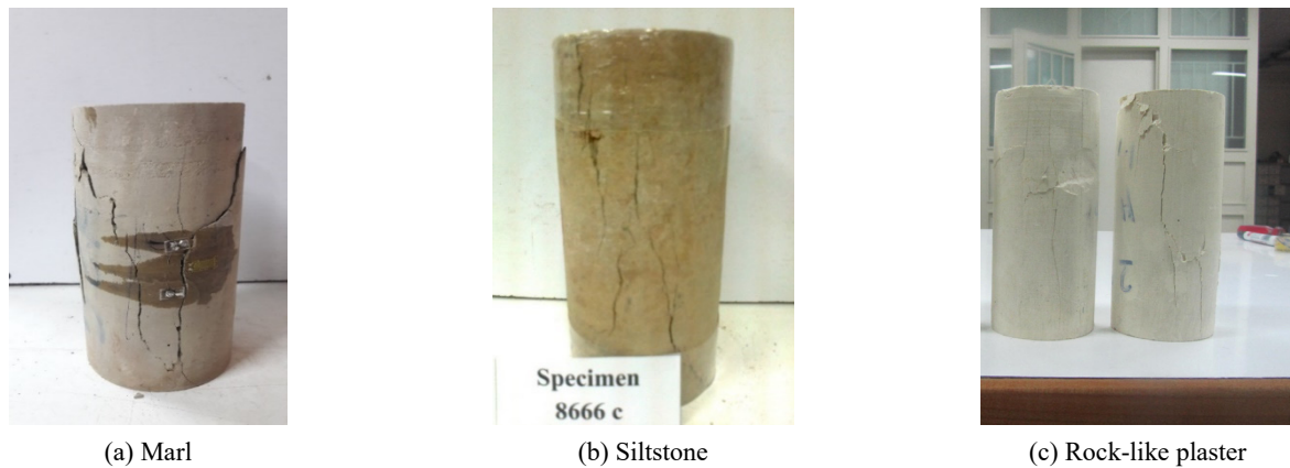
Fig. 4 Spalling-shearing failure mode of low-brittle specimens
