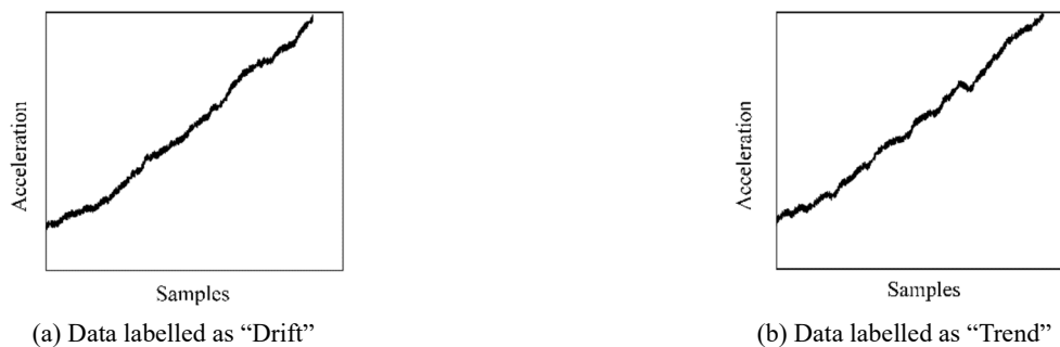
Fig. 4 Selected data readings from a single sensor at different times. No clear distinctive characteristics between the two fault classes are observed.
