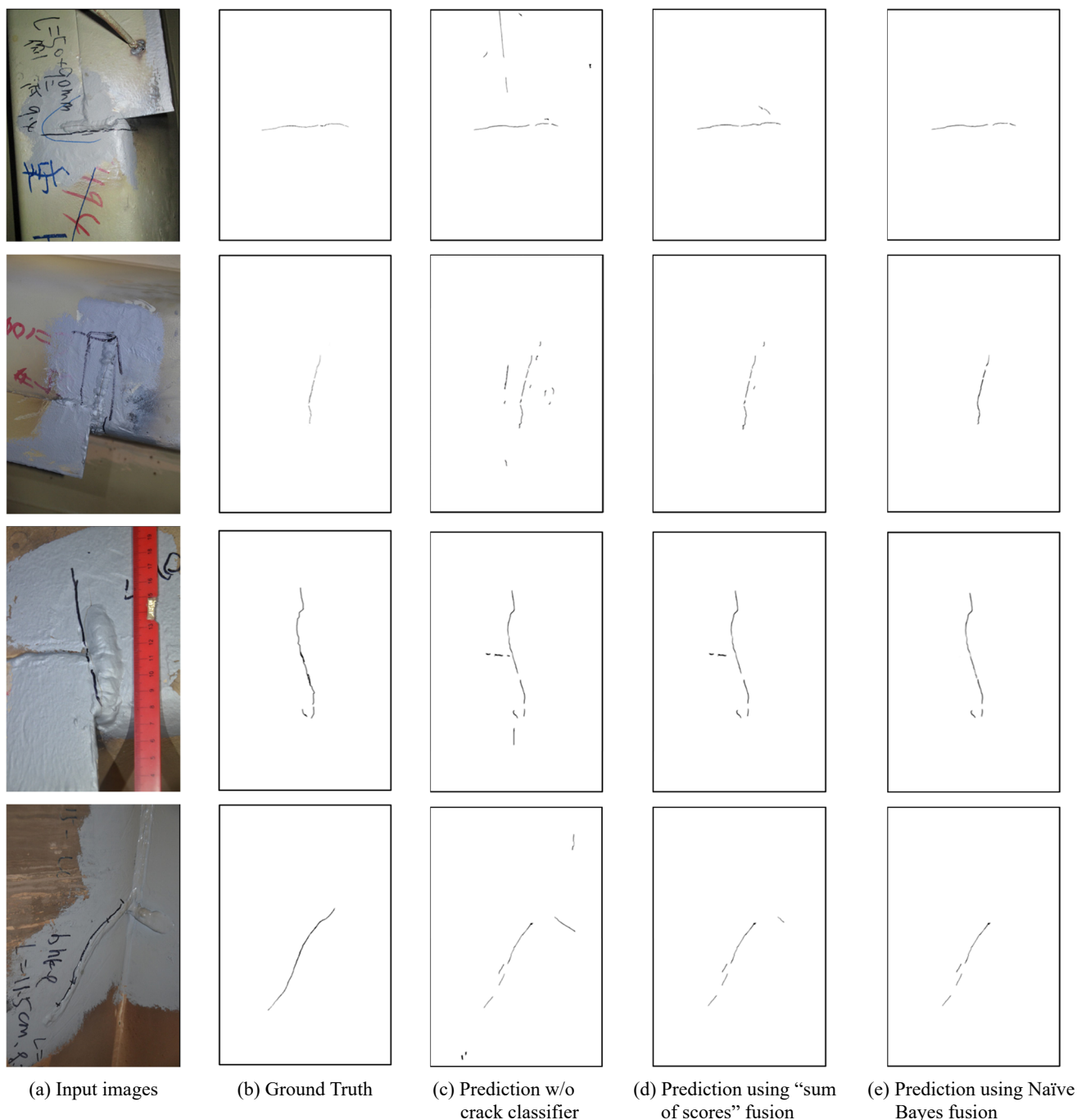
Fig. 12 Sample data and comparison of the predicted crack masks of different configurations.
