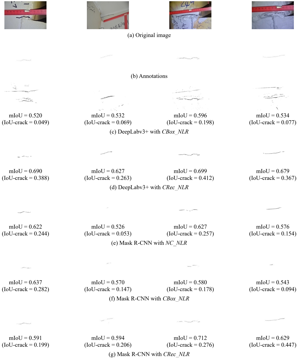
Fig. 9 Demonstration of model predictions on the test dataset with different image cropping strategies and without label refining
