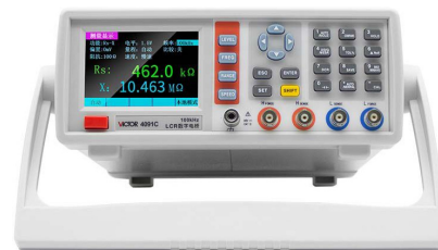
(b) LCR digital bridge tester
