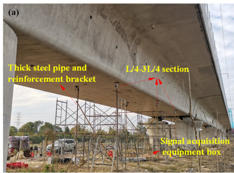
Fig. 11 Layout drawing of the dynamic load testing of the investigated typical 32 m box girder
