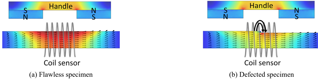
Fig. 1 Magnetic flux leakage phenomenon schematically
