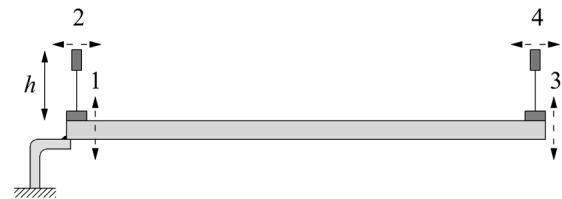
Fig. 16 The location and installation procedure of accelerometer sensors to measure vertical and rotational DOFs
