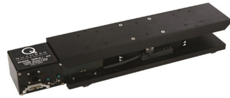
Fig. 8 Shaking table used for experimental test
