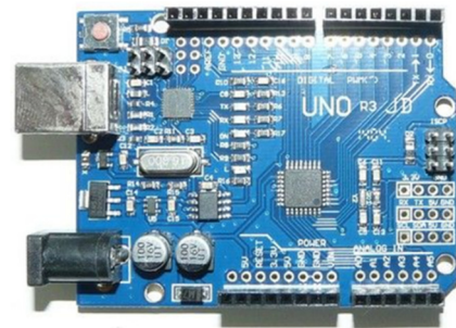
Fig. 6 Controller platform ATmega328
