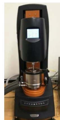
Fig. 6 Discovery HR-3 magnetorheological rheometer used for characterization of MRE
