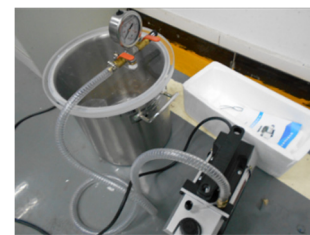
(b) Vacuum equipment
