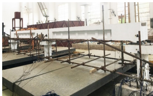
(a) Scaled bridge model with 8 m pier
