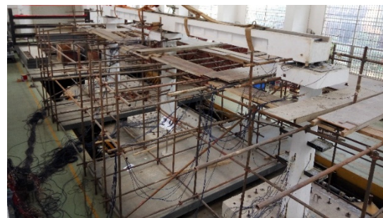
(b) Scaled bridge model with 25 m pier
