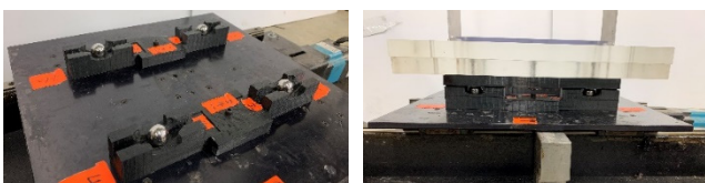
Fig. 14 The 3D printed rolling isolators
