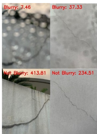
Fig. 5 The variance of Laplacian for blur detection
