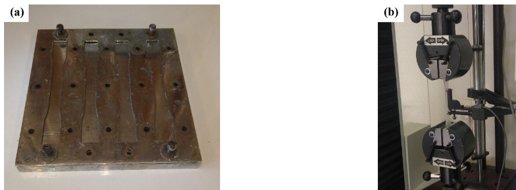
Fig. 2 The general view of tensile specimen mold (a) and test setup (b)
