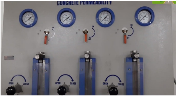
Fig. 1 Permeability water testing tool, water flowing ratio measuring inside the concrete sample
