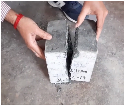
Fig. 8 Measuring the water penetration and cracks
