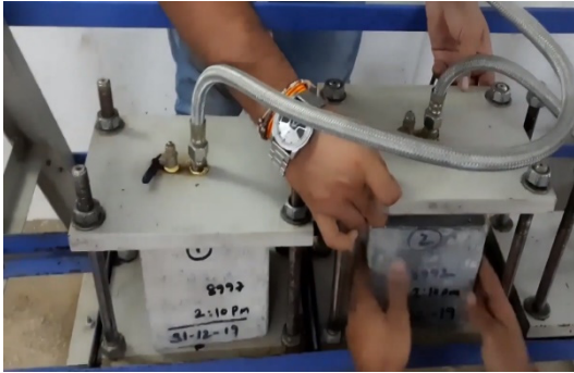
Fig. 3 Placing the samples that were 28 days cured and dried
