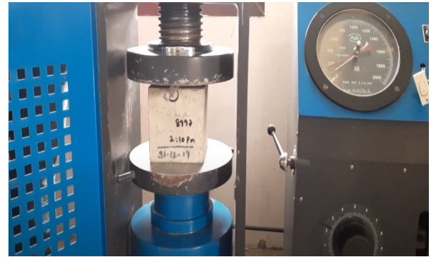
Fig. 6 Immediately split the samples in the plane perpendicular to the face on which the pressure was applied
