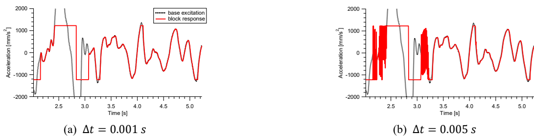
Fig. 19 Effect of time integration step on acceleration response for Coyote Lake comp. 230, \mu = 0.125
