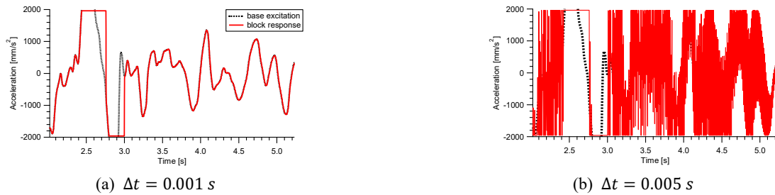
Fig. 20 Effect of time integration step on acceleration response for Coyote Lake comp. 230, \mu = 0.20
