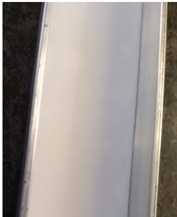
Fig. 7 PTFE sheet bonded to aluminum channel
