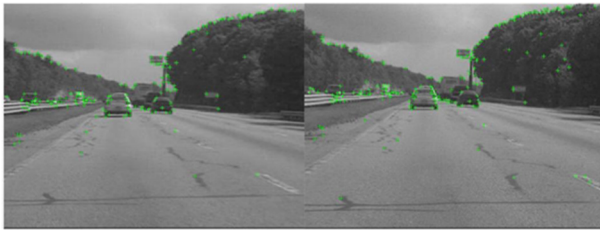
Fig. 8 SIFT point detection
