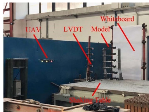
Fig. 14 Setup of the UAV test
