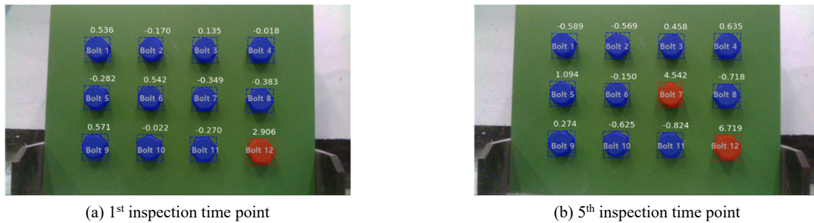
Fig. 14 Identification of loosened bolts for case 4 shown in Fig. 13
