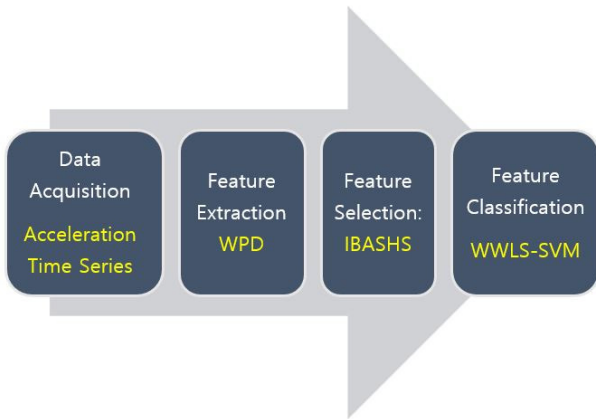
Fig. 1 Summary of damage detection approach
