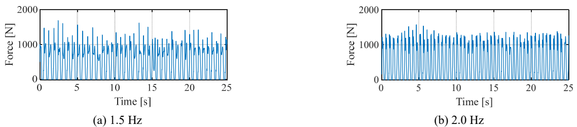
Fig. 3 Individual jumping load records
