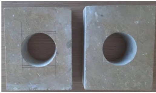
Fig. 4 A central hole of diameter of 7.5 cm and thickness of 6 cm is drilled at the specimens' center
